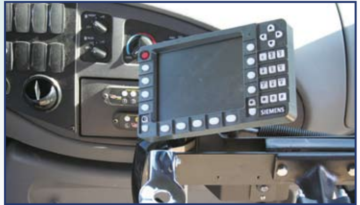
Photo above: The new mobile data terminal (MDT) that will be installed on all of the Handi-Vans.
